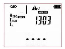
The tester is in autotest mode for Class II devices. Icons displayed on the left side represent all tests that will be performed. On the right side the current time is shown.
