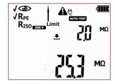
Measurement of PF protective conductor has been completed. If the measurement result is negative, further measurements will not be conducted. In case of the positive test result: If the AUTO-TEST mode is on, the tester will automatically run the subsequent test, which by default is: Riso. If the AUTO-TEST mode is off the tester will wait for the START/STOP button to be pressed. At this stage it is possible to return to the previous test to repeat
