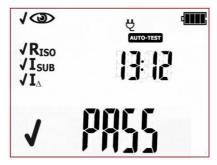
Positive test result for the tested device. The result of each single test of the sequence is positive. Green LEDs of PASS indication are on. On the right side of the screen the current time is shown.
