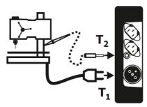
Connection diagram for Class II (III) appliances. The test lead with the probe must be connected to  $\mathsf{T}_2$  terminal socket. The measurement is made between shorted L and N, and the probe:
