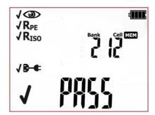
A cell occupied by AUTO test, IEC or PRCD test result (corresponding icons for subsequent tests, along with results are displayed on screen).
