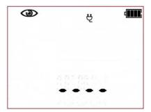
The tester is waiting for the evaluation of the cable's (extension cord) condition after completing visual inspection.
