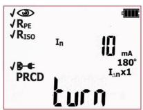
Switch on PRCD. Tester will commence the first measurement. If PRCD trips, a message prompting to switch on the RCD will be displayed on the main screen: 'turn on PRCD'.
