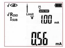
Measurement of RISO insulation resistance has been completed. If the measurement result is negative, further measurements will not be conducted. In case of the positive test result: If the AUTO-TEST
