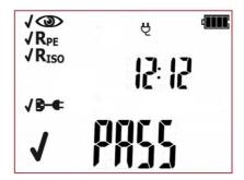
Positive test result for the tested device. The result of each single test of the sequence is positive. Green LEDs of PASS indication are on. On the right side of the screen the current time is shown.
