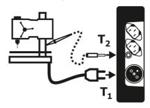
Connection diagram for Class II (III) appliances. The test lead with the probe must be connected to  $T_2$  terminal socket. The measurement is made between shorted L and N, and the probe:
