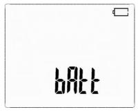
Rechargeable batteries completely discharged.
